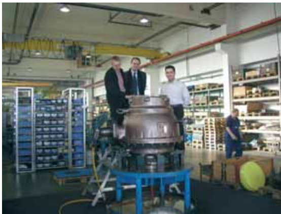
Tightness test - KHSVi 600-VII, AF, KFC, PN 40. From left to right: Mr Marti, KKW Gösgen, Mr Franz Gysi, Franz Gysi AG and Mr Avci from KLINGER Fluid Control, Gumpoldskirchen.
