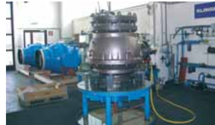
Pressure and tightness test for the whole valve and the drain valve. Certification and approval acc. to EN10204-3.1B of all parts incl. bolts and nuts.
